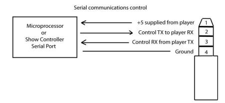
The SS-38 can supply 5V DC at up to 100 mA, from Sprite 1, to power your micro controller.
