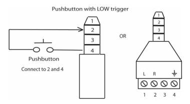
The Control Mode should be set to Trigger Low No Interrupt or Trigger Low with Interrupt or Trigger Low Delayed. No Interrupt and Delayed will queue from the end-of-file on Sprite 1 only.
