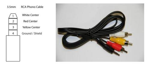
If you get a cable elsewhere, check to see that the wiring is the same. We have seen some cables where the red, yellow and white RCA are wired to different poles on the 3.5mm plug.
