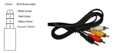
If you get a cable elsewhere, check to see that the wiring is the same. We have seen some cables where the red, yellow and white RCA are wired to different poles on the 3.5mm plug.
