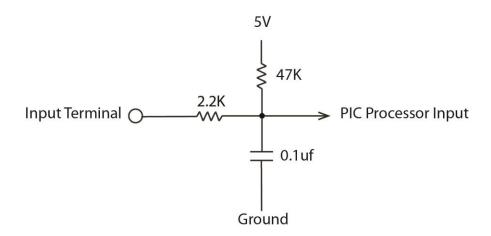
The Hydra input terminals 0 through 9 have a 2.2K series resistor to help limit current flow to a safe level for the PIC processor. There is a 47K pull-up resistor to bias the inputs to a High state. There is a 0.1uf capacitor to help reduce stray noise.
