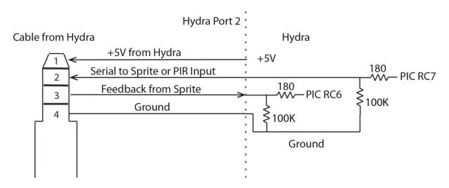
The Hydra Port 2 can be used for a second Sprite or as an input for a motion sensor or other trigger. The use depends on the operation Mode that you select from the table on page 4.
