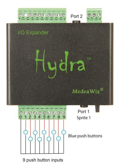
Each pushbutton should have 2 terminal connections.
