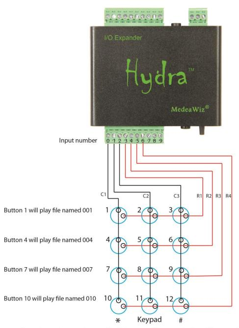
Keypads vary by manufacturer. The Columns and Rows may be in a different order than shown.
