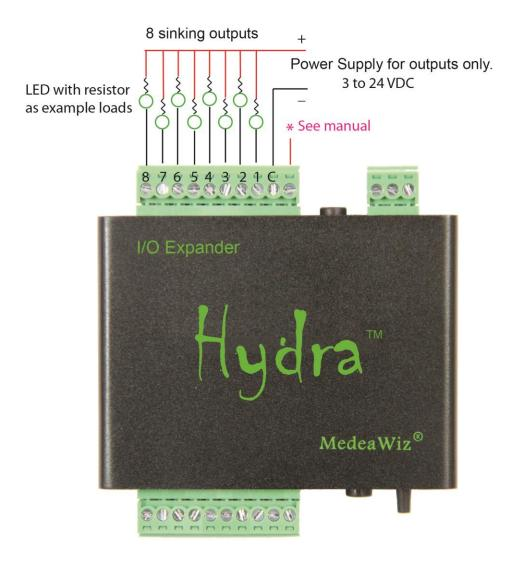
The Hydra has "sinking outputs", which means that it switches the Ground or "Minus" side of the power supply. In this case you will connect the Positive "Plus" of your external power supply directly to all output devices. The Negative "Minus" side of each output device will connect to one of the output numbers 1 through 8 on the Hydra.
