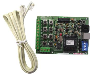
**CAUTION:** Analog touch screen used with DV-66U is subject to any dimension of the standard 4-wire resistive type touch screen; it is different with the matrix type touch screen built in the DV-66104 unit
